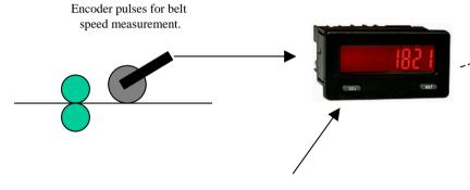
DC power required. If the MLPS1000 is used then this could be mounted in the ENC8B000 enclosure. The MLPS1 is a 85-250Vac power supply that mounts on the rear of the CUB5. This can power the CUB5 and the encoder.
