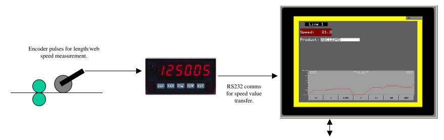
Ethernet port to transfer log directly into Excel. The log is stored in a CSV format to allow simple transfer of data.
