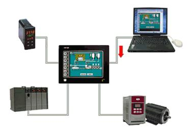
With the G3's powerful protocol converter, you have the ability to exchange data between any and all connected devices. With a few clicks of the mouse, you can map a setpoint from a PLC to a variable speed drive, or provide a PLC program with information as to the status of a PID controller.
